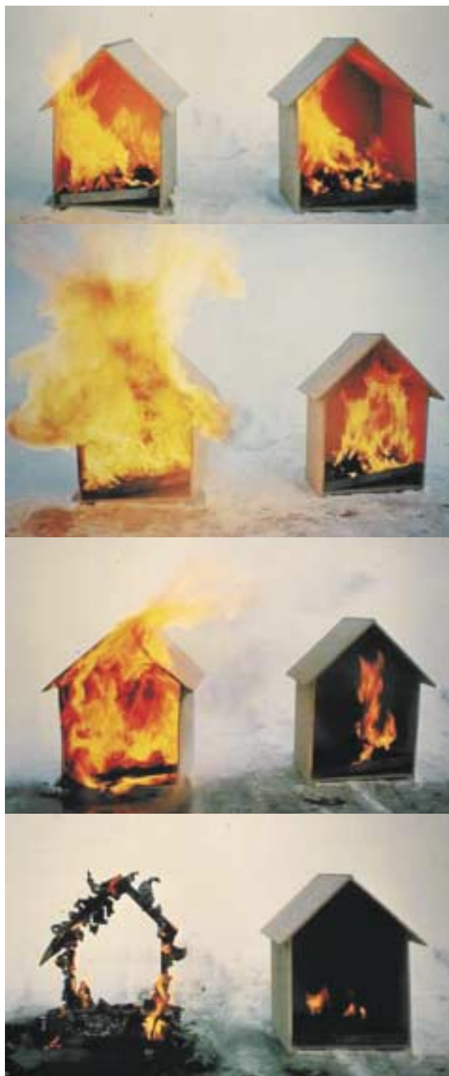
"Dog houses" made of conventional chipboard and Cement Bonded Particleboard
