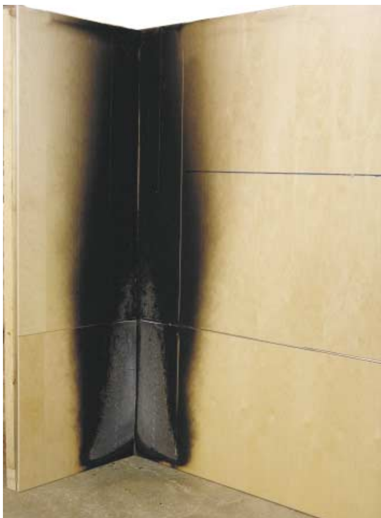
Elam panel in SBI (Single Burning Item)-test
